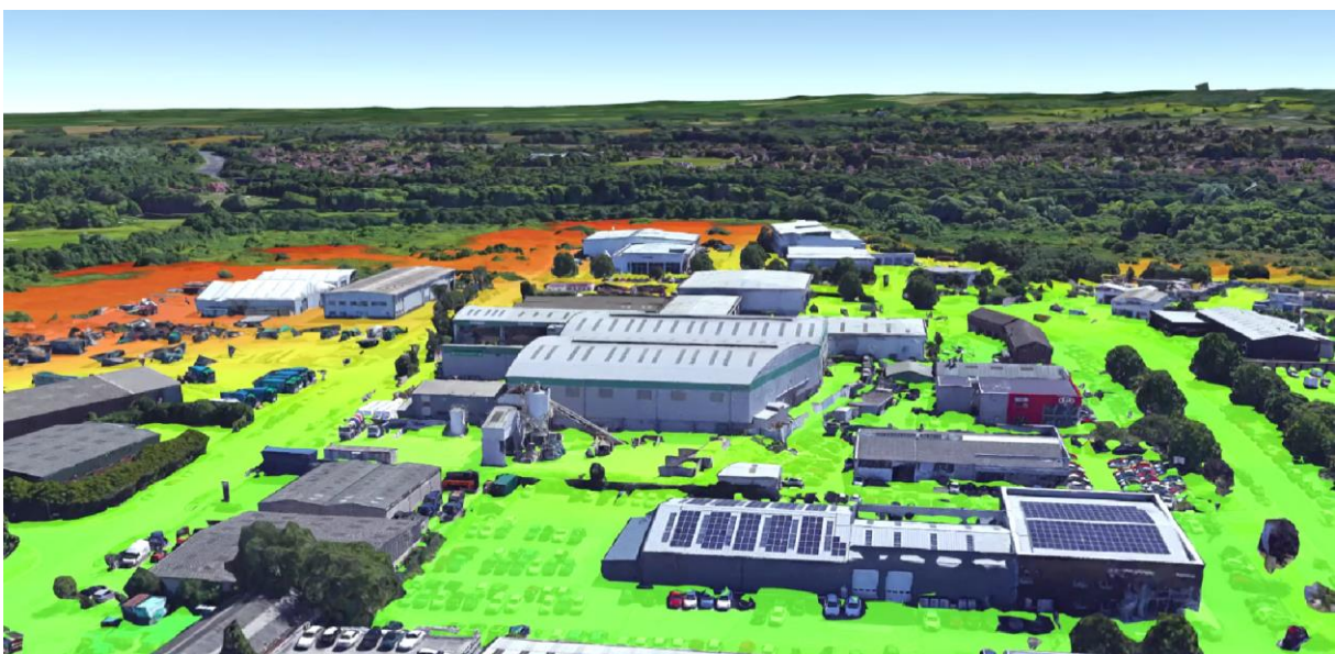
Figure 10. Ground surface vertical velocity (mm/year) presented as coloured pixels on a 3D surface model
